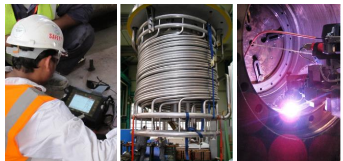
Examples for welding and testing supervision in a cement factory (l), consulting and production of a heat exchanger (m), procedure qualification for the application of deposition welding (r)
