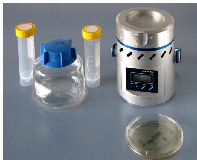
Equipment for taking samples for water analysis and bacterial indoor air measurement
