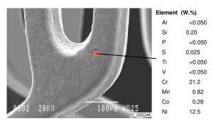
Full quantitative chemical analysis of a very small sample. The diameter of the analysed area is about 5  $\mu m$
