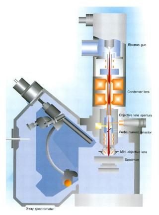
Principle of electron beam microanalysis
