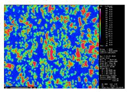
Elemental distribution image of the element nickel in a sintered sample of a nickel/chromium alloy
