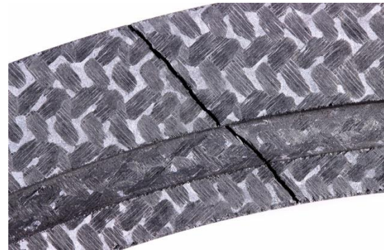
Fracture in a carbon fibre reinforced component
