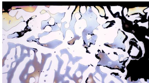
Selective corrosion on a duplex steel pump housing in a flue gas cleaning system (light microscopy)
