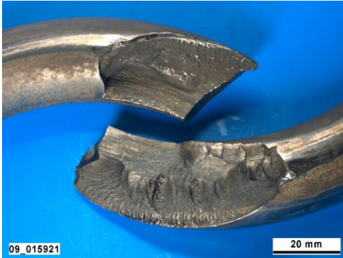
Broken compression spring, spring steel A local surface defect led to crack formation
