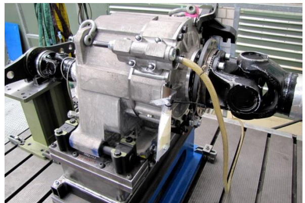
Component fatigue - gearbox under test
